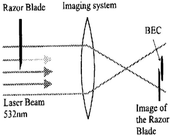
Apply  $\pi$  phase shift to half of the condensate wavefunction with a far detuned Laser beam
