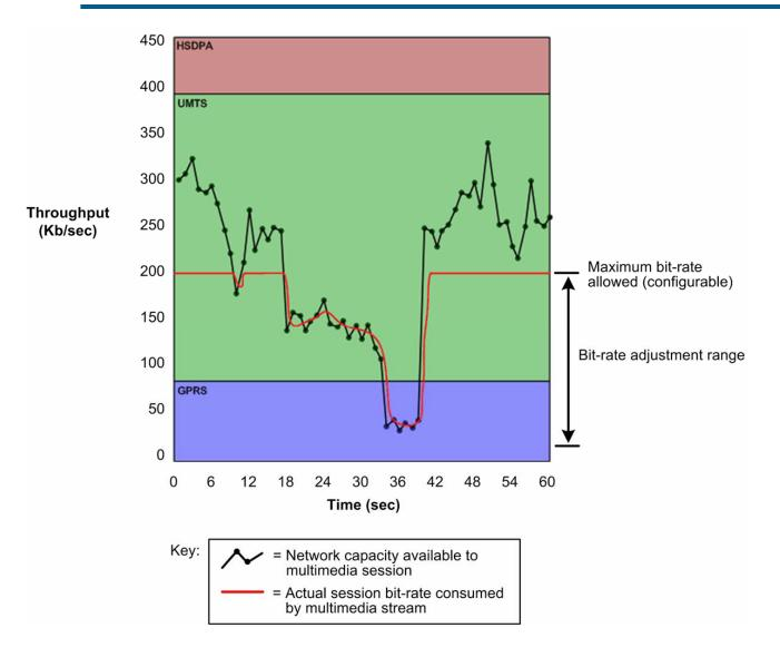
Media function constantly monitors the network connection with the client and shapes the multimedia stream to adapt to current network conditions.
