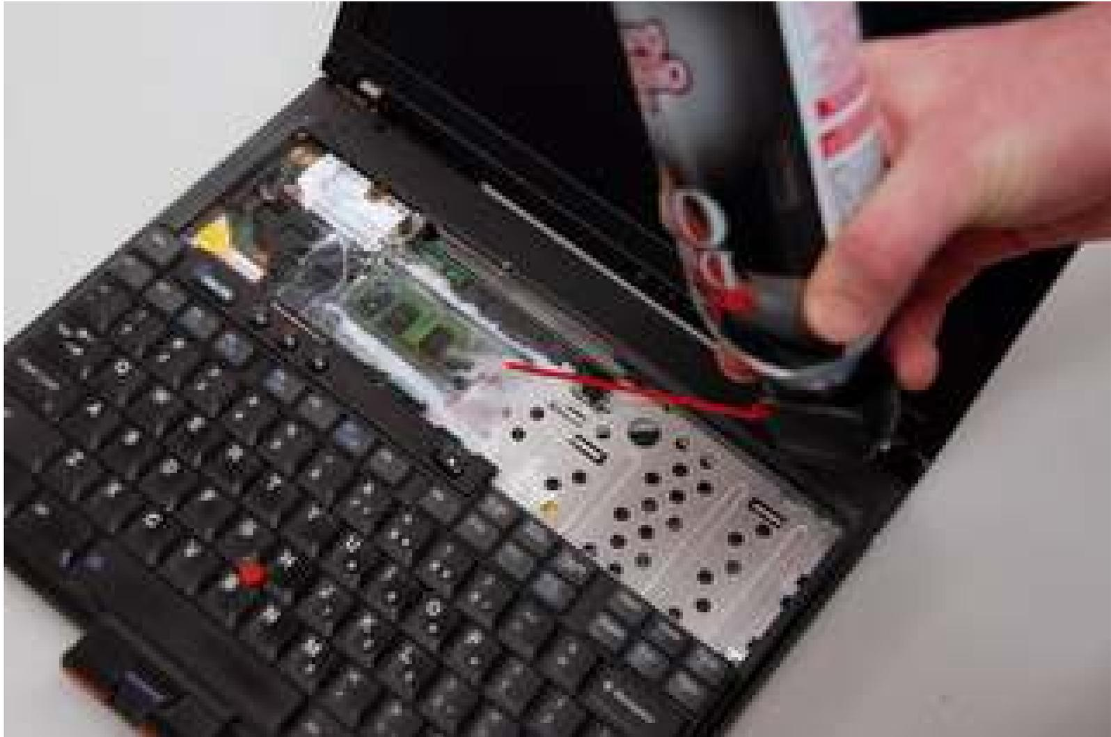
Data can be kept alive for many seconds in unpowered RAM by cooling it with a cheap can of Quick-Freeze:
