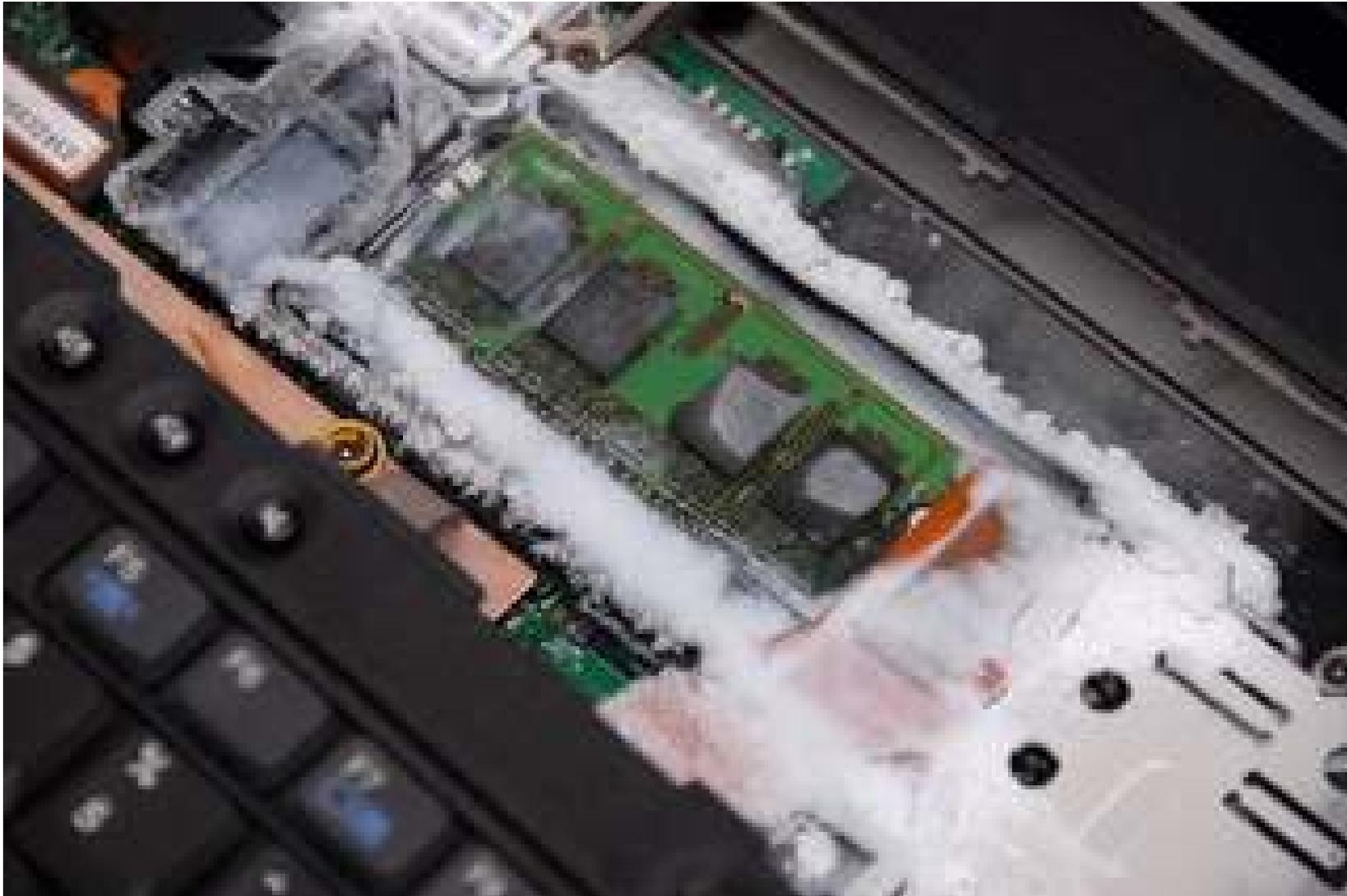
Data can be kept alive for longer periods by using liquid nitrogen:
